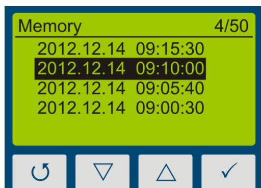
Select the measurement with the keys  $\nabla$ -key and  $\Delta$ -key. Confirm with  $\checkmark$ -key. Return with  $\circlearrowleft$ -key.
