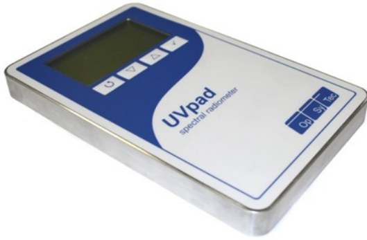
Figure 5. Mobile spectral radiometer with an array spectrometer in a Czerny-Turner variant.
