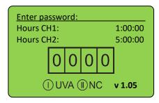
Even without PIN the operational hours, connected sensors and firmware version are displayed. After entering PIN and confirmation with OK you can change system settings:
