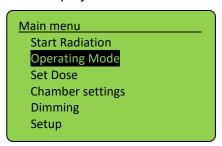
The menu items in the main menu depend upon the settings, i.e. the menu items "Dimming" and "Irradiation time" are only displayed, when the respective mode has been selected.
