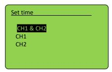
Now you can select the decimal with the keys  $\triangleleft$  or  $\triangleright$  and with the keys  $\triangle$  or  $\nabla$  you can set the time to the desired value. Confirm with OK ( $\checkmark$ ) to return to the main menu.
