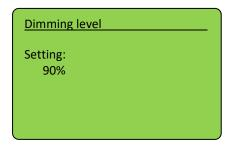
Use  $\triangle$  and  $\nabla$  keys to set desired value. Confirm with  $\checkmark$ .
