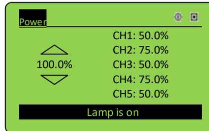
The status screen displays the current powers, the set operating mode, the internal or external control and error messages.
