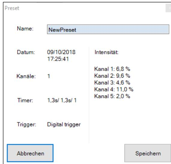
In the "Preset" window, the settings with which the preset is saved are displayed. Before clicking the Save button, the name of the preset must be set. The preset name may only be used once and must not contain a space, semicolon or line break.
