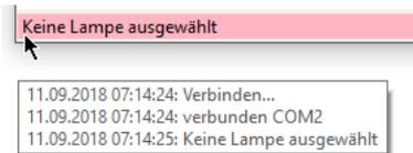
Errors and messages appear in the display for 3 s, errors are highlighted in red. The last ten messages are displayed here when the mouse pointer hovers over them.
