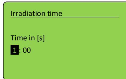
Here, the decimal place is selected with the ◀ or ▶ key and the time is set to the desired value with the △ or ▽ keys. Confirm with OK (✓) to return to the timer main menu.
