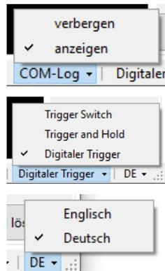
The COM log area can be made invisible here by "COM log" -> "hide" and visible again by clicking on "show".
