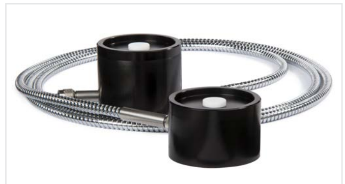
Optical fiber and external sensor (type 1 background, type 2 front)
