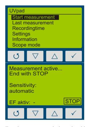
From the standby menu, a measurement is started with the key ✓-key.
