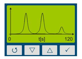
With the key  $\nabla$ -key, the profile of irradiance for UVA, UVB UVC and VIS is displayed.
