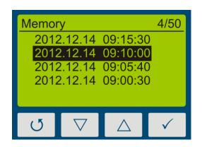
Select the measurement with the keys  $\nabla$ -key and  $\triangle$ -key. Confirm with  $\checkmark$ -key. Return with  $\circlearrowleft$ -key.
