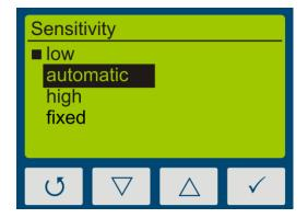
In the setting "automatically", the UVpad adjusts the sensitivity, once a minimum irradiance is existent. This setting is suitable for most applications.
