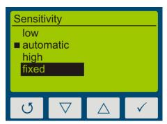
Step 3 To adjust the integration time press the  $\nabla$ -key or the  $\triangle$ -key.
