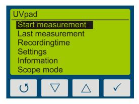
In the standby menu, the UVpad is switched off via the key O-key.
