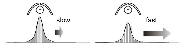
At high speed and a low lamp power, a higher integration time is required. Thus, the UVpad might possibly not measure directly underneath the UV lamp, but integrates (averages) this range. The displayed irradiance is then minimal lower. With the continuous measurement performed, the dosage is not affected.
